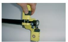
Push cable cutter over the cable and fix it with locking screw so that all rolls are placed.
