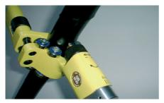
For the final radial cutting place back the blade in position "0" and turn the tool around the cable.
