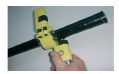
For stripping process rotate the tool around the cable. The blade cuts in the sheath spirally.
