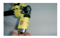
By lifting the disk adjustment of the cutting speed is done. Position 2 for cutting the outer jacket, position 1 for cutting the insulation and for large diameters of uter jacket.
