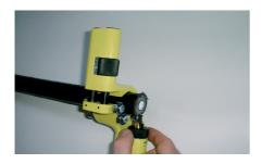
Adjust the cutting depth of the blade. A cutting depth by approx. 80% is enough. This is avoiding damages of the screen wires or the cable core.
