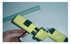
To cut and remove the insulation slip on the plastic insert.
