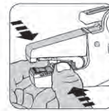
Squeeze wire stopper from both sides
